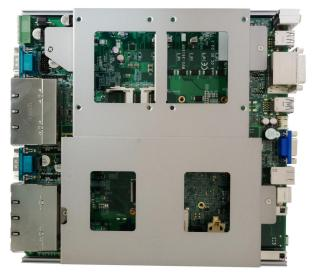
Unscrew four M3 F-head screw on SATA HDD bracket and then remove it.
