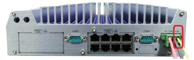
To have ignition power control for in-vehicle usage, you need to supply IGN signal to Nuvo-3616VR series. The IGN input is located on the back panel via a 3-pin pluggable terminal block (shared with DC power input). Here is a general wiring configuration for in-vehicle deployment.
