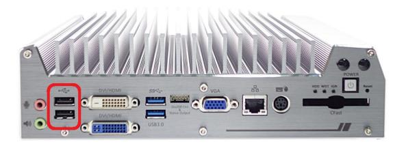
In addition to two USB 3.0 ports, Nuvo-3616VR series provides another two USB 2.0 ports on the front panel. By BIOS default, these USB 2.0 ports are operated in EHCI (Enhanced Host Control Interface) mode and are compatible with USB 2.0, USB 1.1 and USB 1.0 devices. Legacy USB support is provided so you can use USB keyboard/mouse in DOS environment.
