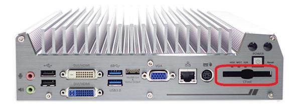
Nuvo-3616VR series provides a CFast socket on the front panel. CFast is a new interface for portable storage device. It shares a similar form-factor as CompactFlash but leverages Serial ATA interface to offer higher data transfer rate. The CFast socket on Nuvo-3616VR series is a push-push type. You can insert and push a CFast card to the end to install it, and push the installed CFast card again to eject it.
