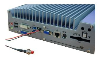
3. Push the non-latched switch will turn on the system (the PWR LED indicator on the front panel is on at the same time). Push the non-latched switch when system is on will turn off the system. If your operating system supports ATX power mode (i.e. Microsoft Windows or Linux), push the power button causes a pre-defined system behavior, such as shutdown or hibernation.
