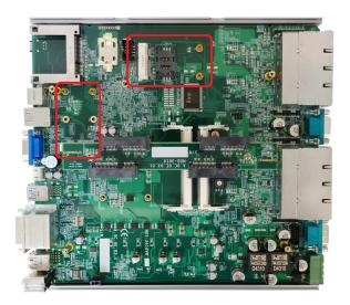
2. Tilt the mini-PCle WIFI module and insert it to the mini-PCle connector. And fix the WIFI module with two M2.5 P-head screws.
