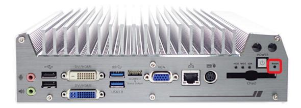
The reset button is used to manually reset the system in case of any abnormal condition. To avoid unexpected operation, the reset button is hidden behind the front panel. You need to use a pin-like object to push the reset button.
