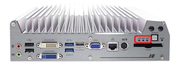
There are three LED indicators on the front panel: HDD, WDT and IGN. The descriptions of these three LED are listed in the following table.
