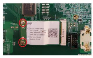
3. Attach the IPEX-to-SMA cable to the WIFI module and fix the SMA connector (on the IPEX-to-SMA cable) to the SMA antenna aperture on the back or front panel.
