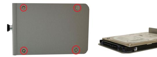
Gently slide the HDD tray assembly into the slot on the side of Nuvo-3616VR till it's firmly connected to SATA connector.
