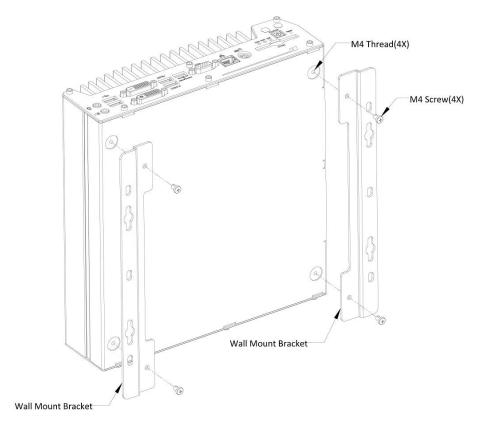
2. Place Nuvo-3616VR series on the wall or on a flat surface and fix it with screws. You can also take advantage of the keyhole-shaped holes of mounting brackets to suspend Nuvo-3616VR series on the Wall.
