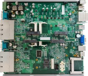
5. Unscrew two M3 P-head screws and then remove the mezzanine board.
